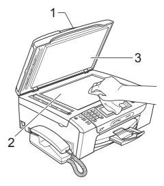
In the ADF unit, clean the white bar (1) and the glass strip (2) with a lint-free cloth moistened with a non-flammable glass cleaner.
